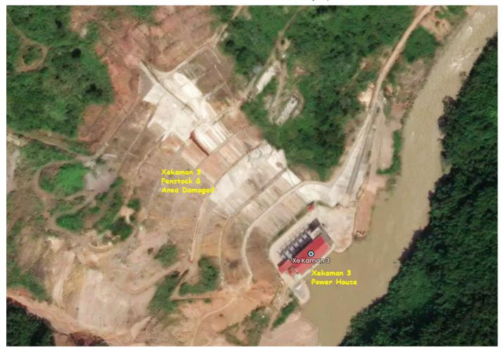
Penstock damage December 2016 - Fairly soon after completion, the Xekaman 3 power plant started to be plagued by landslide problems at the penstock which appears to have been constructed on an ancient landslide slope. Problems started soon after the reservoir was filled as small land displacements caused major damage to the penstock and associated pipelines. At one location it appeared that a sinkhole was opening up and there also may have been a new channel being formed.
