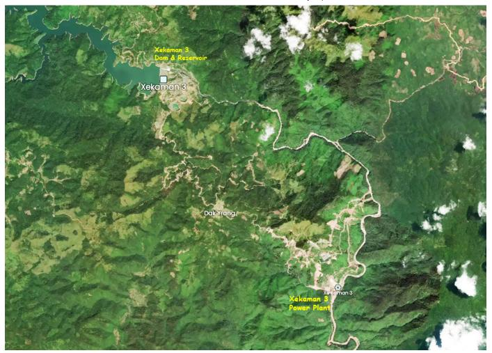
The reservoir surface full supply water level is 960 meters above mean sea level with low supply level at 925 meters above mean sea level. Active storage volume is 108.5 million cubic meters.
